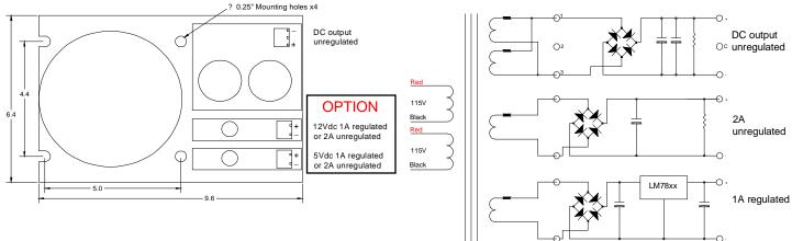
AC power connections: 115Vac – 2 red wires to neutral & 2 black wires to hot. 220Vac – 1st red wire to hot, 1st black wire to 2nd red wire, and the 2<sup>nd</sup> black wire to hot. Ground connects to chassis.
