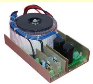
These power supplies are used for stepper, servo motor drive and high over loaded applications. They will work on both standard 115V and 230V at 50Hz or 60Hz. This Toroidal transformer has heavier gauge wires then the normal requirement to avoid the copper lost during the full load output and over load output.
