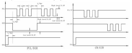
Figure 10: Sequence chart of control signals
