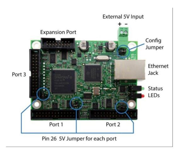
An external 5V power source needs to be connected to the green power terminals on the ESS. For G540 or other breakout board configurations, the Pin 26 5V Jumpers should be OFF for Ports 1, 2, and 3, and 5V should be supplied to the External 5V Input.
