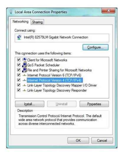
Select the "Use the following IP address" button, and then configure the settings as shown below. IP Address should be 10.9.9.1, subnet mask should be 255.255.255.0:
