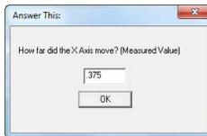
Measure the amount the machine actually moved and input here.
