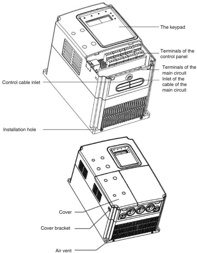
Figure 1-2 Parts of inverter( 15kw and below)
