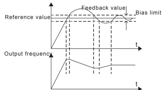
Figure 6.23 Relationship between bias limit and output frequency.
