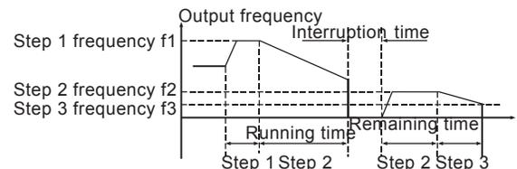
Figure 6.26 Simple PLC continues from interrupted step.
