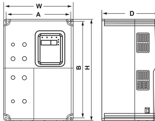
**Figure A-1 Dimensions (15kW and below) (380V)
