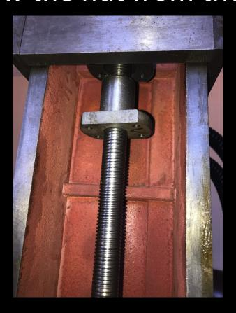
You can now pull the lead screw out of the top block. If the bearing comes with it. Put it back in the block
