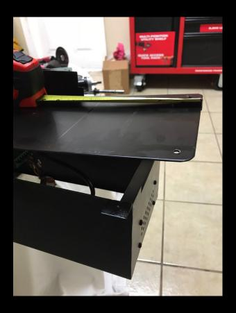
I am taking 5 ½" off the bottom. You can remove up to 9". There are two tapped holes with nothing in them. Use that as I guide for how much you can safely remove.
