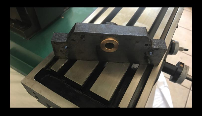
Then you can start to slide the table off of the Y axis saddle.
