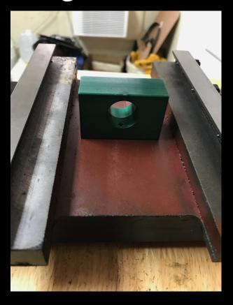
Make sure the ball nut, and the threaded end of the ball screw are on the right hand side of the machine.
