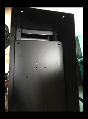
There are 6 screws on the inside piece of sheet metal. You can remove these and slide the sheet metal out far enough to remove some of it.
