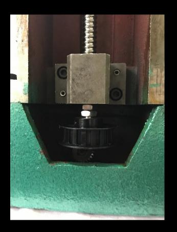
Slide the ball screw up through where the old lead screw nut was. The end of the ball screw will go into the existing bearing of the top block
