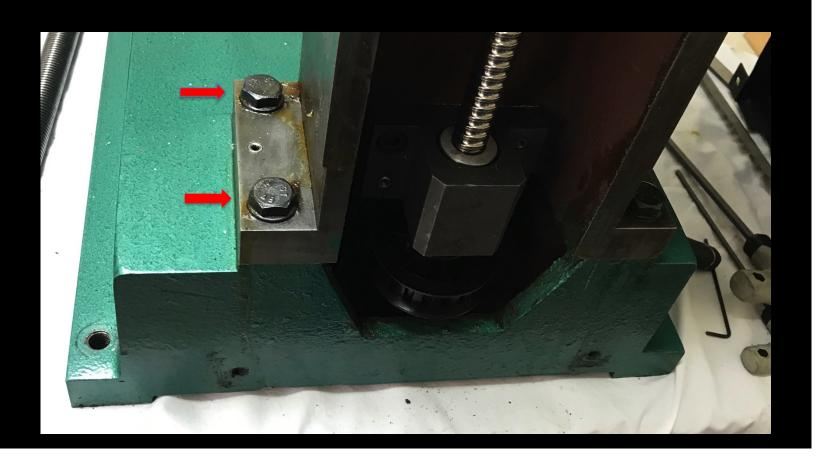
Use cap screwed supplied with the kit for the brackets. The old bolts are not long enough.
