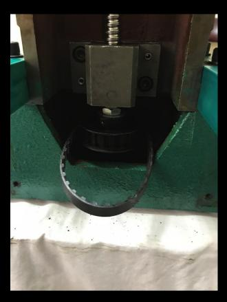
Rotate the ball screw until the ball nut block snugs up against the upper plate where the old lead nut was.
