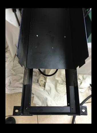
Now you can install the back cover and slide the motor mount through.
