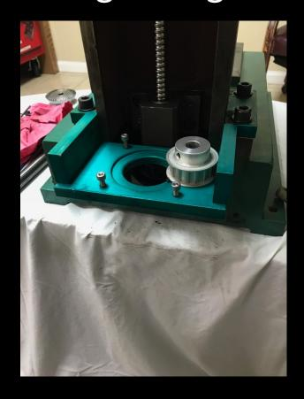
• The pulley in the last picture installs onto the motor shaft. Make sure you have good alignment of the two pulleys to keep the belt level. The motor plate is slotted and adjusts in and out to put tension on the belt.
