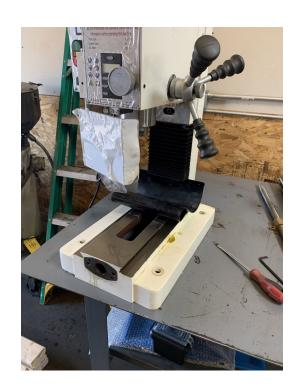
We found the best way to handle Z is to lay the machine back onto the column. Then remove the cover plate.
