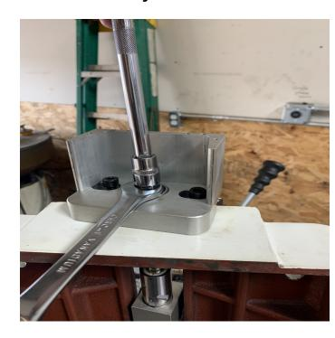
Set the machine back upright and slide the saddle back on. Be sure to slide the gib back in as well and put the retaining screw back in
