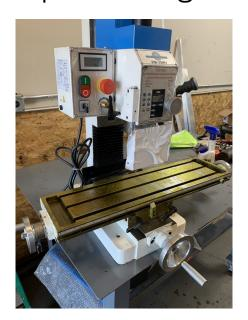
Start with removing the handles. Make sure and take the key out as well.
