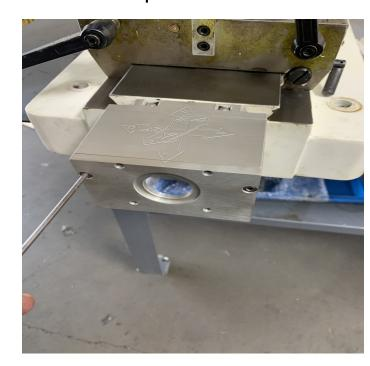
Bolt down the X ball nut block to the existing tapped holes.
