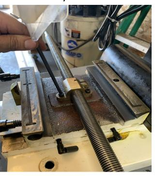
Moving to Y. Remove the two cap screws behind the hand wheel Also remove the two cap screws for the way cover. Crank the handle and unscrew it
