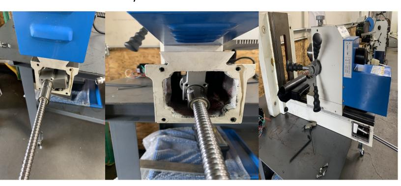
You will need to set the plate and install the motor at the same time. It is easiest to put the coupling on the motor first, then the whole thing slides onto the end of the ball screw.
