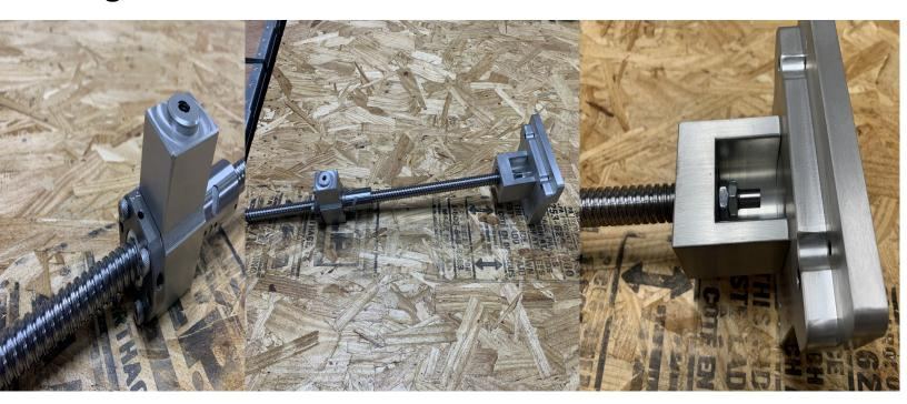
Make sure the cap screws are tight and slide the Z assembly into the column
