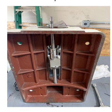
Drop the Y motor mount onto the shaft with the bearings installed and tighten down the jam nuts
