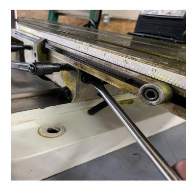
Bolt on the bearing plate and tighten down the jam nuts. Bolt on the motor mount
