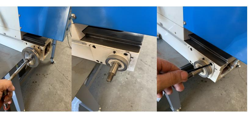
There are two gears that need to be removed. Remove the set screw from the first one. You can then pull out the backing plate and push it off the shaft.
