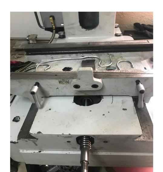
Bolt down the block with this cap screw. We had the front of the base off the bench to get a hand underneath to line it up.
