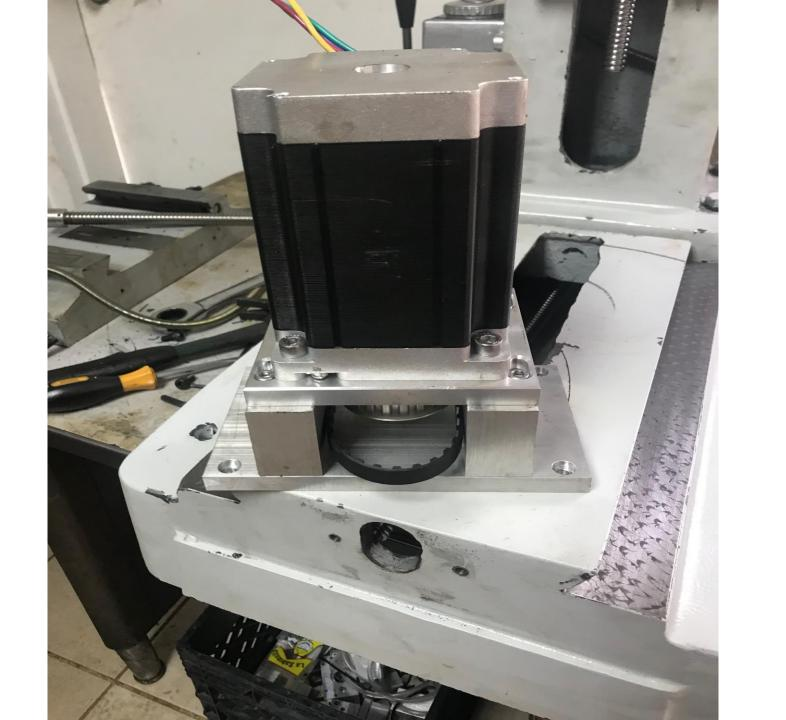
The motor plate is slotted for tightening the belt. We had to use a timing belt due to the location of the ball screw. It is so far forward it would cause interference to try and make it direct drive.
