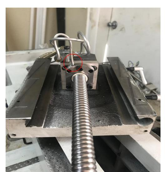
Now you slide the Z saddle onto the ways. It just barely fits. You could also grind away the corners at the bottom of the ways just a bit if it doesn't quite fit.
