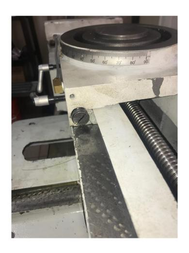
Bolt on the bearing block and tighten the jam nuts Now is a good time to check alignment, and get everything sliding back and fourth smoothly. It's easier to do while the column is laying down on
