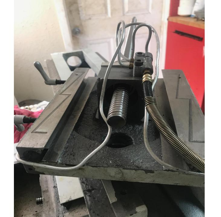
The one free oil line will go into the tapped hole on the ball nut. Be sure to position the ball nut accordingly
