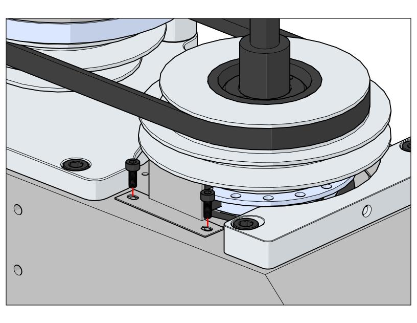
Reinstall the spindle index sensor, and make the electrical connection. You may need to open up the holes slightly for mounting. The hole location from the manufacturer has been known to vary quite a bit. Some customers have had to add their own tapped holes, but in most cases you should be just fine.
