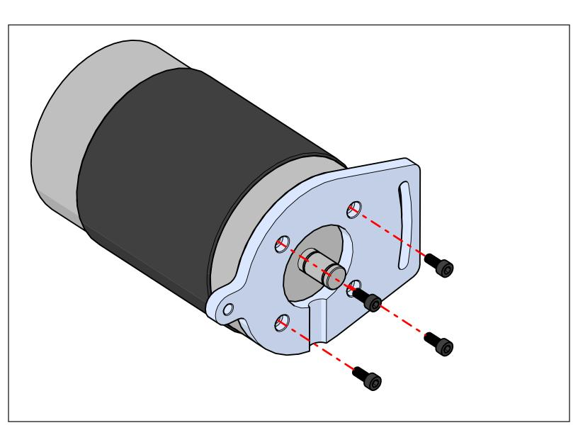
Mount the motor plate to the motor. Mind the orientation of the motor so that your power wires can be ran appropriately.
