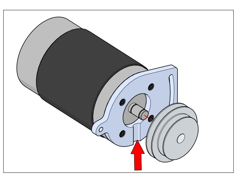
Mount the motor pulley onto the motor. There are two setscrews 90° apart that lock the motor pulley in place. The groove machined in the motor plate is to allow you to make adjustments of the motor pulley. You may just want to snug these for now as you will probably need to adjust the pulley to make sure it's in line with the spindle pulley.
