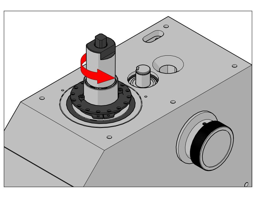
Remove the spindle cap that retains the drawbar. Some machines are equipped with a small hole in the spindle nose that you can put a bar in to keep the spindle from turning. If your machine doesn't have it, you may need to use a strap wrench around the nose of the spindle. Generally these caps aren't very tight and are pretty easy to remove.
