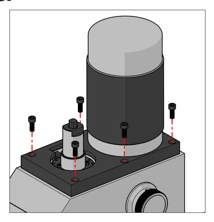
Remove the six M6 socket head cap screws so that the motor and mount can be removed as one assembly. Depending on your machine you may have to disconnect the motor power wires. Be sure the machine is unplugged before doing so to prevent injury.
