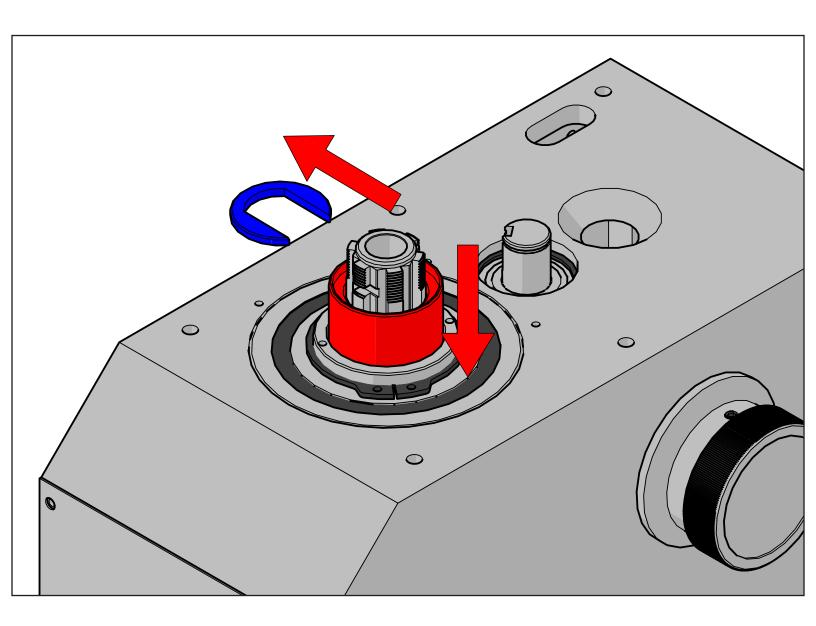
This step requires two parts. First you need to compress the spring cup (red) down far enough to expose the spindle c-clip (blue). I've found using a flat blade screw driver to press down on the spring cup works well. Then slide the c-clip out. Lastly remove the spring cup.
