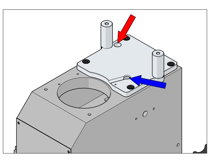
The red arrow is where the motor power wires come through. The blue arrow is where the RPM sensor wires are ran thru the channel machined in the bottom of the plate. This step is for the Optimum BF20 mill only.
