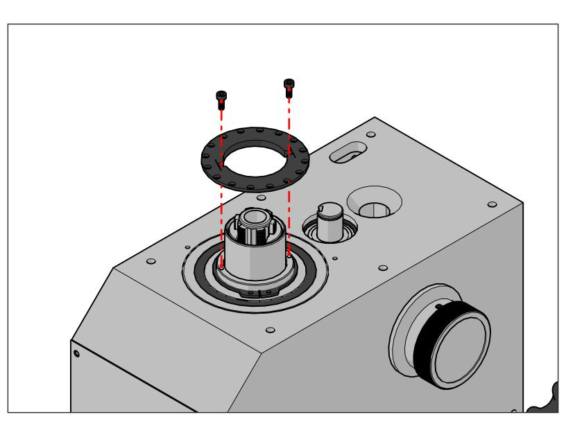
Remove the two socket head cap screws fixing the index ring to the stock drive gears and remove the index ring. If you have the Optimum BF20 skip this step and move to the next.
