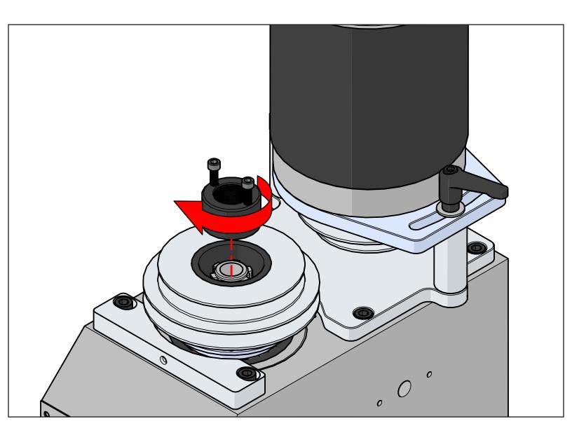
Install the supplied (2) o-rings to the spindle nut and then thread into place using the two socket head caps screws to help aid gripping the nut. Once the nut is installed remove the two cap screws.
