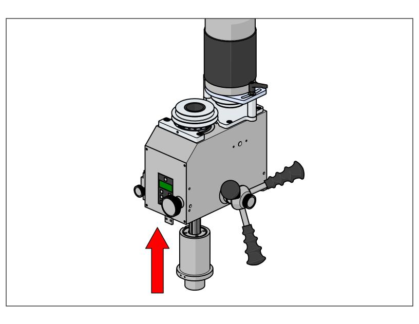
Reinstall the quill and spindle assembly, brass quill pin, quill locking handle and lastly the spacer between the quill body and the DRO unit.
