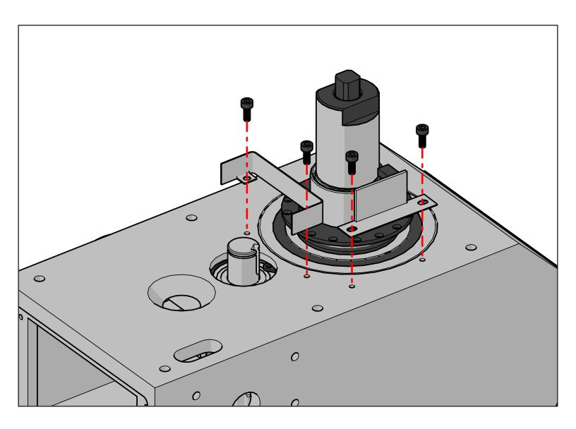
Next disconnect the spindle RPM sensor plug and remove the two screws holding it in place. Remove the other two screws holding the grease guard in place. Set these two items aside. If you have an Optimum BF20 machine your sensor is a proximity and uses magnets to pickup the spindle RPM. The optical sensor shown here uses an idex ring with holes in it. Etiher way remove the mount for the RPM sensor.
