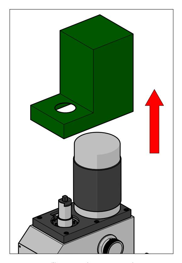
Start off by removing the motor cover as shown.
