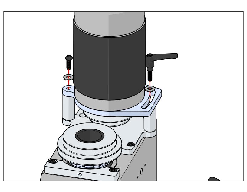
After you are happy with the alignment of the pulleys, add the hardware as shown to fasten the motor in place.
