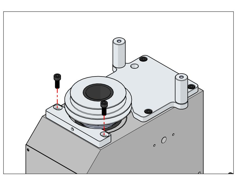
Mount the belt cover bracket. The mounting holes are slotted to allow adjustment for centering the belt cover on the head.
