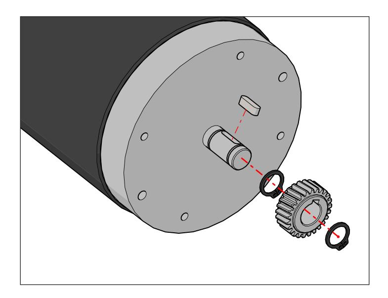
After removing the motor from the base, next remove the first snap ring, then remove the gear from the motor shaft. A small puller may be necessary if the fitment is tight. Next remove the second snap ring. Lastly remove the drive key.
