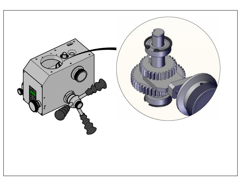
The next step is to remove the intermediate gears. These are the ones that break when you have a spindle failure. This shot is basically outlining the sub-assembly. There are two snap rings, upper and lower. They both will need to be removed. Some versions of the machine have the snap rings and some don't. If you have them, you'll need to remove them.
