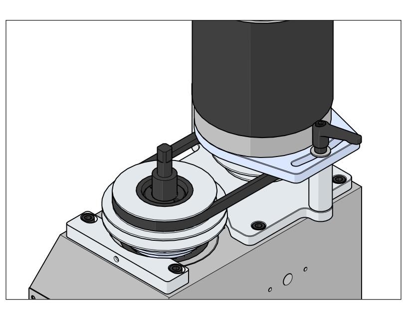
Install the belt and apply tension.
