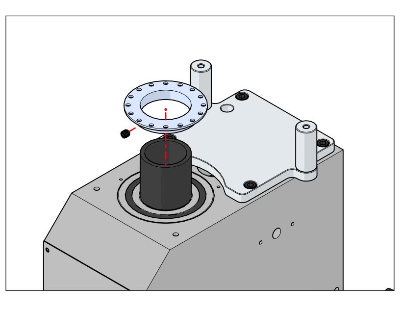
Slide the index ring over the bearing carrier seating it against the upper bearing, then tighten the setscrew to secure the ring in place. Make sure the setscrew is being applied to the flat machined on the bearing carrier. A thread locker such as Loc-Tite wouldn't be a bad idea either. If you have the Optimum BF20, then this step doesn't apply to you, go ahead and skip this step.
