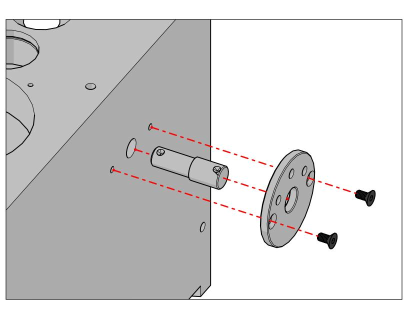
Remove the two flat head screws, followed by the detent flange, and lastly the selector shaft.
