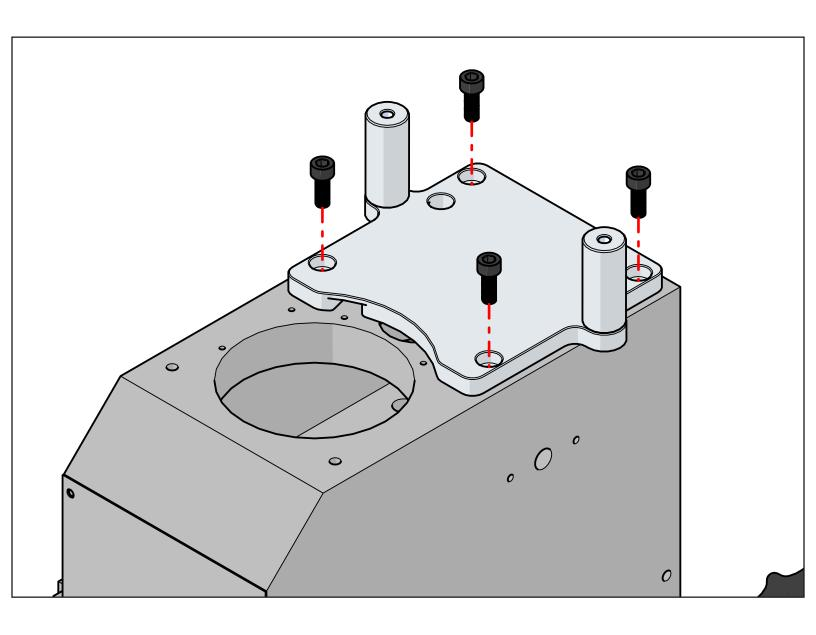
Mount the baseplate to the head using the stock M6 socket head cap screws.
