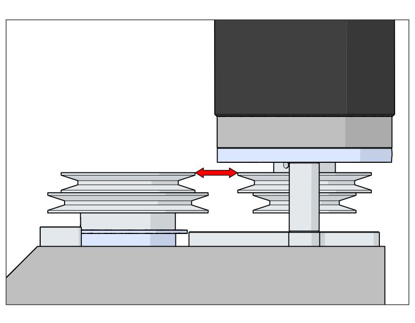
Next temporarily set the motor on the standoffs and make sure the two pulleys are in line. If you need to adjust it, do so before fastening in place.
