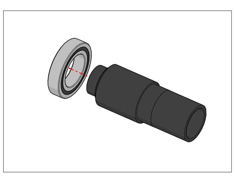
Press the lower bearing on the bearing carrier. Take caution not to damage the bearing. If you don't have a press, use a soft face mallet or a soft piece of metal such as aluminum or brass. Never strike the bearing directly with a hammer. If you have a press, either arbor or hydraluic, this would be the prefered method to press the bearing on. Do not put the upper bearing on yet.
