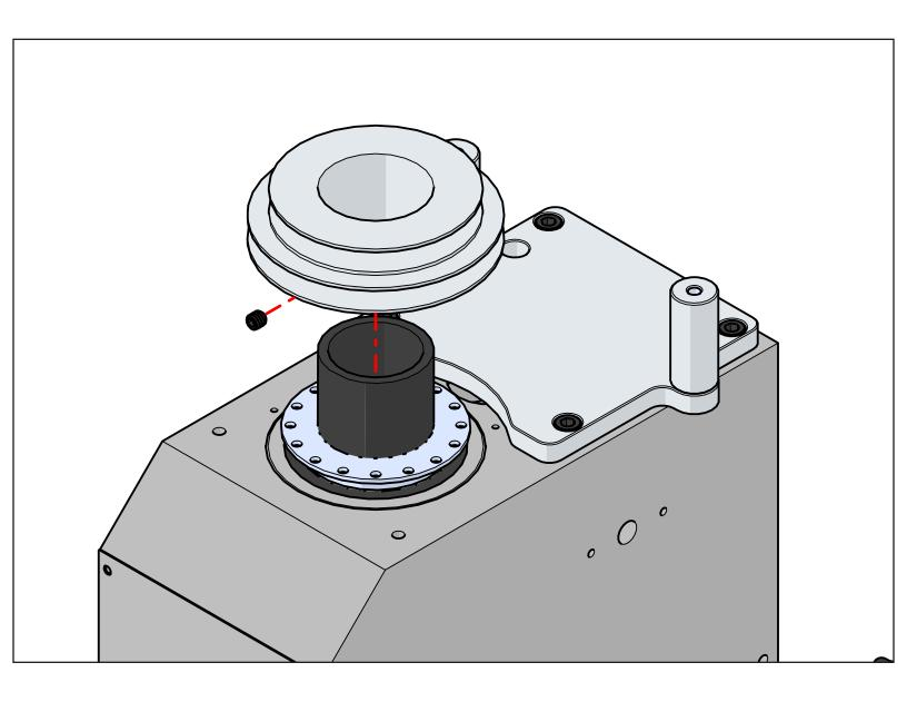
Slide the spindle pulley over the bearing carrier and tighten the setscrew to secure the pulley in place. Again, Loc-Tite is a good idea here. If you have the Optimum BF20 your pulley will have a slighty longer shoulder that has magnets for the proximity sensor. However it mounts the exact same way.
