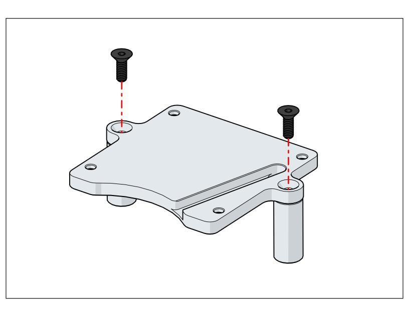
The first step is to mount the motor standoffs to the baseplate using the provided M6 flat heads. If you have the Optimum BF20, your baseplate will have a different wire channel on the under side, but the standoffs mount the same.
