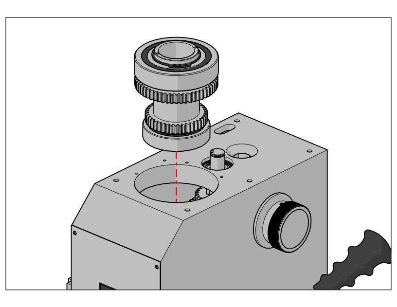
Remove the drive gear sub-assembly out through the top of the head. Use a soft material like aluminum, brass or even wood and hit the assembly upward. It will typically come out pretty easy.
