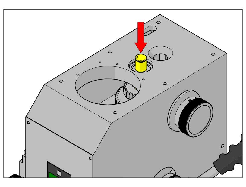
After removing the snap rings, drive the intermediate shaft (yellow) out through the bottom of the head. The shaft will slide through the intermediate gears leaving them loose inside the head casting.
