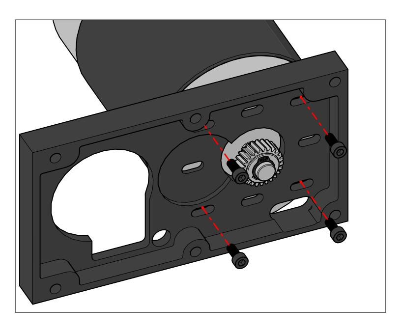
Remove four M5 socket head cap screws holding the motor to the base.
