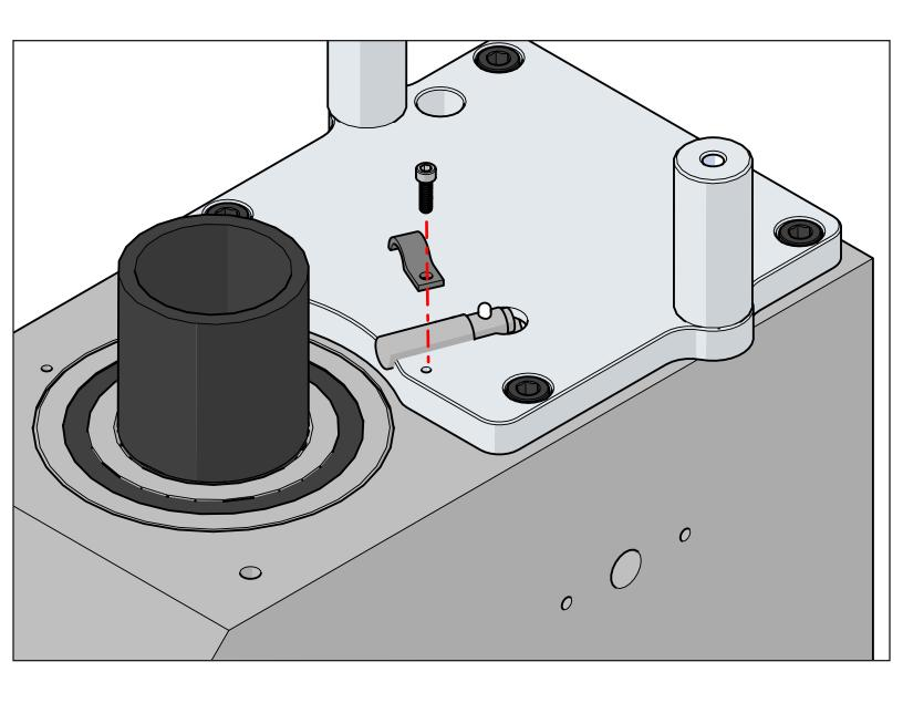
Mount the spindle proximity sensor with the supplied clamp and socket head cap screw. This step only applies to those with the Optimum BF20.
