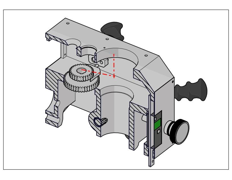
Remove intermediate gears and selector fork through the top of the head as shown.
