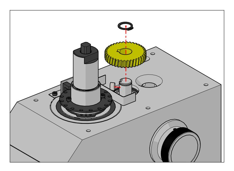
Once the motor and base have been fully disassembled, set them aside. Next we need to remove the intermediate gear that's attached to the intermediate shaft. This is done by removing the snap ring, then removing the gear from the shaft. Lastly remove the drive key.
