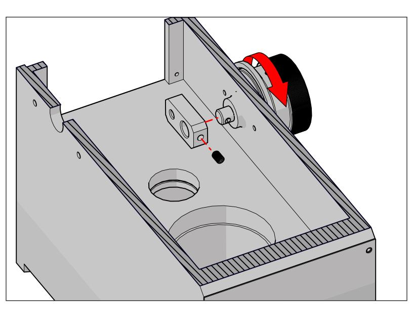
This step is optional, if you wish to leave the gear selector knob in place then skip these last few steps. You don't NEED to remove this as it won't interfere with the new belt drive kit. If you wish to remove the knob you first need to remove the selector arm from with inside the head. Rotate the selector knob so that the set screw is facing forward, then remove it.
