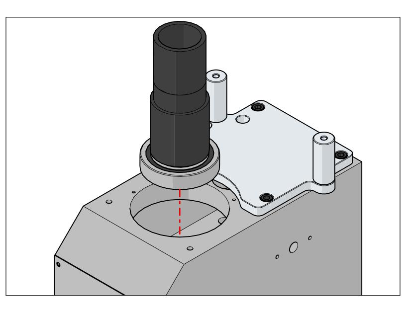
Take the bearing carrier with the bottom bearing pressed in place and seat it into place. Again use a soft face mallet, or soft metal such as aluminum or brass to seat the bearing carrier in the head. Be sure the carrier is seated the whole way down.
