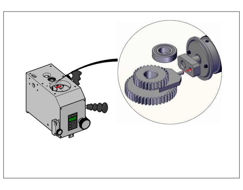
Slide the gear and fork from the speed selector arm.
