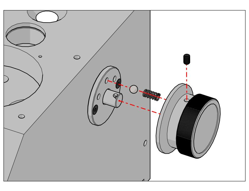
Remove the set screw fixing the knob to the shaft, remove knob. Be aware of the detent spring and ball behind the knob.
