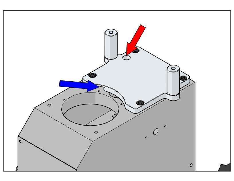
The red arrow is where the motor power wires come through. The blue arrow is where the RPM sensor wires are ran thru the channel machined in the bottom of the plate. If you have the Optimum BF20 your baseplate is different because it uses a different sensor for to pick up the spindle RPM. Please move to step 28b. if the Optimum BF20 is your machine.
