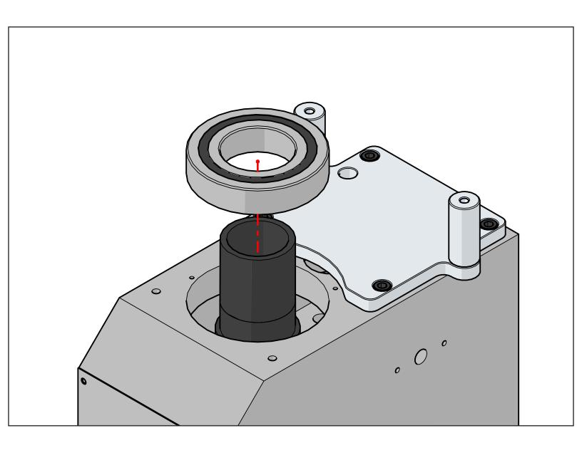
Now drive the top bearing into place. The bearing should be flush with the top of the head when fully seated.
