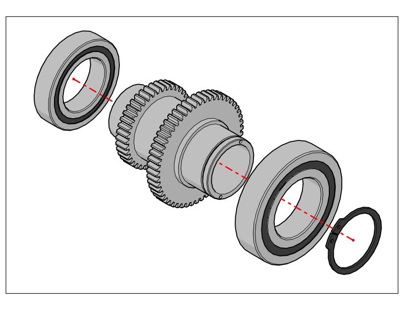
If you purchased the bearing kit with your belt drive kit, you can skip this step and move onto the next. If you decided to re-use the exisiting bearings, then you need to remove them from the stock drive gears to be re-pressed on the new bearing carrier that is supplied with the belt drive kit. This is probably the hardest part of the disassembly as the bearings are known to be quite difficult to remove at times. The easiest way, is to use a gear puller. Be careful not to damage the bearings.
