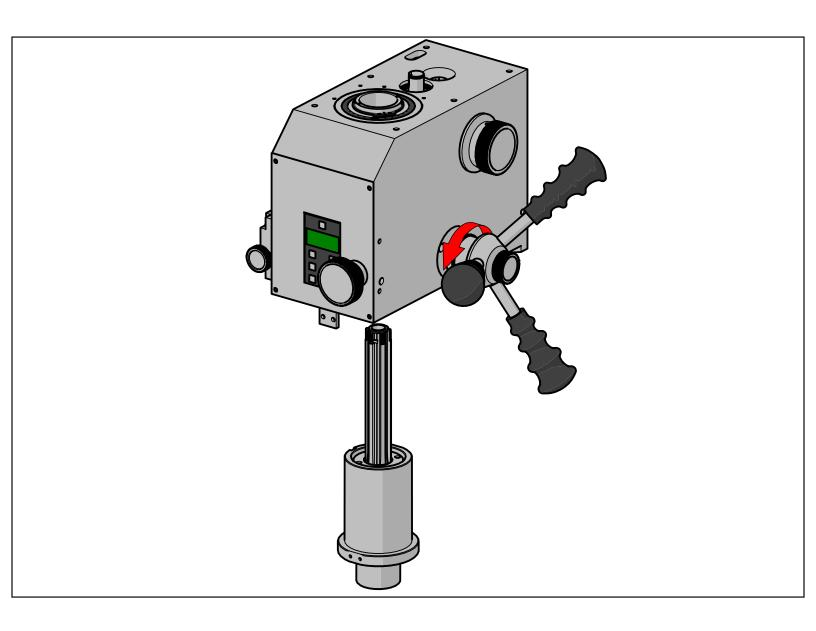
Remove the DRO block from the spindle. Rotate the quill handle to lower the quill and spindle assembly out the bottom of the head. Set quill/spindle assembly aside.
