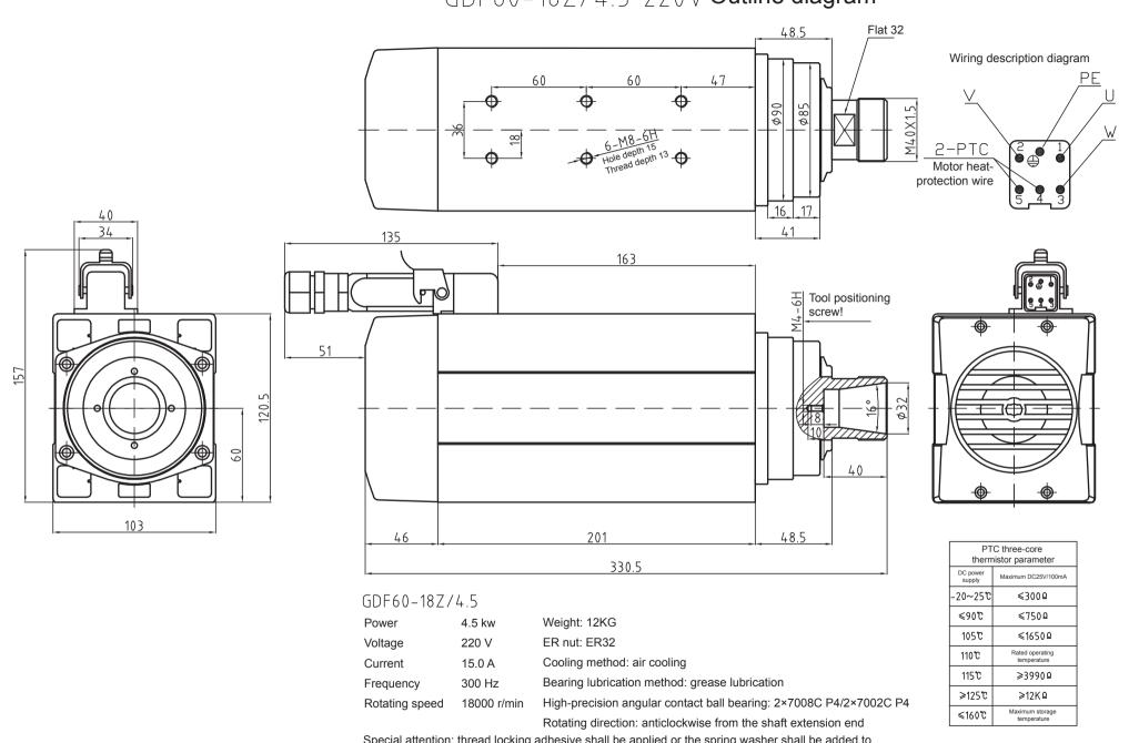
Special attention: thread locking adhesive shall be applied or the spring washer shall be added to prevent the looseness during the installation of the fastening screw!
