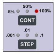
Press CONT button to select Continuous jogging mode. Press STEP button to select Step jogging mode.
