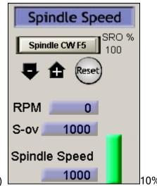
Press SPINDLE + button to increase Spindle OverRidden (SRO) each time. Press SPINDLE - button to decrease SRO 10%.
