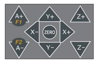
In STEP mode, press and release jogging button to move selected axis one step with selected step size.
