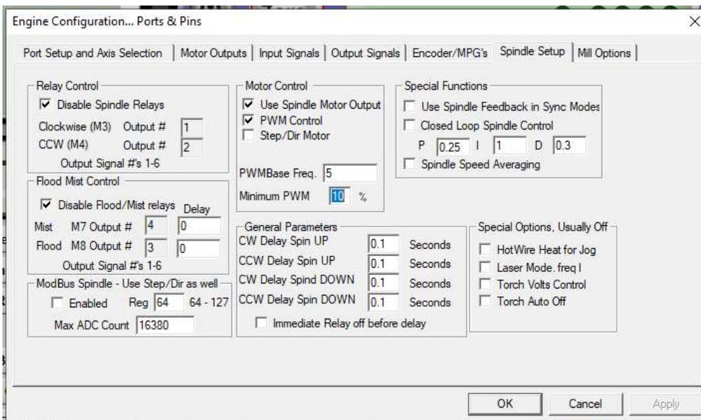
Check off “Disable Spindle Relays”. The Output 1 Inhibit still works because of the spindle settings under the motor outputs tab Spindle Step being set to port 14, which is output 1.
