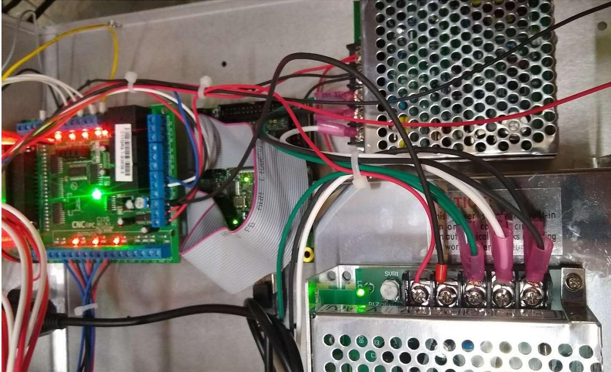
Note that in the photo on the 12V PS, V- is connected to the GND terminal of the 0-10V section
