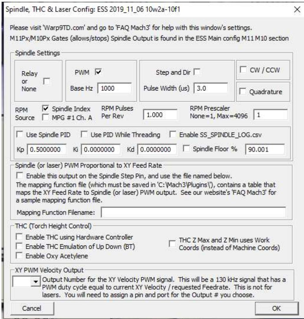
This screen is under “PlugIn Control” Menu” PWM must be selected, Step/Dir will not work.
