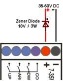
For lower <u>limit</u> switches of the device, one can lead full output voltage of plasma source. In this connection <u>do not connect anything to the other input</u> <u>terminals of the controller.</u>
