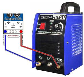
When connecting directly, use the shortest possible cables for connecting the plasma source with THC controller - it is recommended the THC controller to be located directly at the plasma source.
