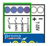
The relay outputs "Arc, Up, Down", are controlling outputs via relays, and should not be utilized for anything other then it's intended use.
