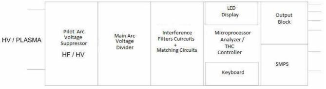
Pilot Arc Voltage Neutraliser - protection system, which is responsible for removing spikes in the AC electrical flow, which can be caused by a plasma source with contact-less arc striking (HV/HF pilot arc) generating a high voltage or from surges coming from plasma cutters equipped with contact arc striking system.
