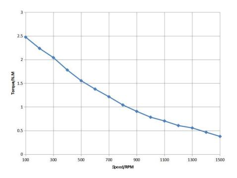
Test condition: 36VDC Power supply, KL-5056 Stepper Driver, Drive Current: 5.6APK, Microstep: 1600
