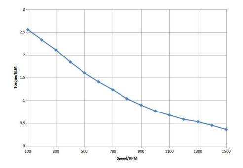
Test condition: 36VDC Power supply, KL-5056 Stepper Driver, Drive Current: 4.9APK, Microstep: 1600
