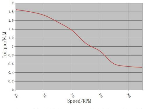
Test condition: 36VDC Power Supply, KL-5042 Stepper Motor Driver, Drive Current: PK3.41A, Microstep: 1/8
