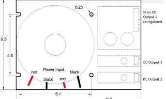
This power supply is designed for used in the step/servo motor drive and high over loaded applications. It will work on both standard 115V and 230V at 50Hz or 60 Hz. This toroidal transformer has heavier gauge wires then the normal requirement to avoid the copper lost during the full load output and over load output.
