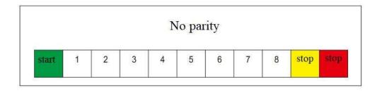
In above picture, the starting signal of a single data packet for serial communication is represented by logical 0 data bit, and the two stopping signals of data packet are represented by logical 1 data bit.
