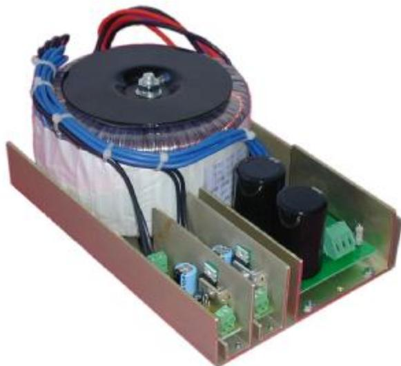
These power supplies are used for stepper, servo motor drive and high over loaded applications. They will work on both standard 115V and 230V at 50Hz or 60Hz. This Toroidal transformer has heavier gauge wires than the normal requirement to avoid the copper lost during the full load output and over load output.
