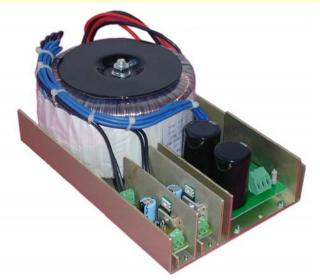
This power supply is designed for used in the Step/Servo motor drive and high over loaded applications. It will work on both standard 115V and 230V at 50Hz or 60Hz. This toroidal transformer has heavier gauge wires then the normal requirement to avoid the copper lost during the full load output and over load output.
