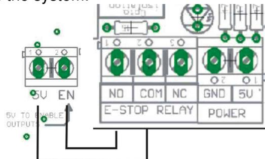
Basic connection of the E-STOP RELAY. For more advanced connections check:
