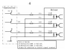
Figure 3: Connection to PNP signal (common-cathode)
