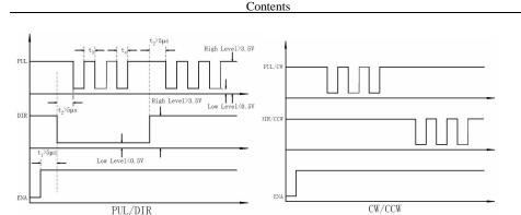
Figure 10: Sequence chart of control signals
