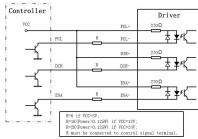
Figure 2: Connections to open-collector signal (common-anode)
