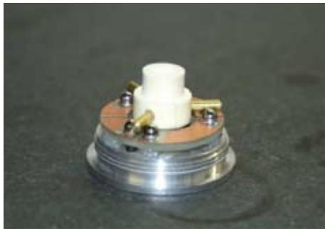
The movable contactor is made from a hard polyester resin plastic with 3 brass rods. Three brass rods are molded into the plastic and extend out from the plastic piece 120 deg
