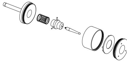
The shaft is a hardened steel shaft screwed into the top cap. This is removable to convert it to a tool height setting pad.
