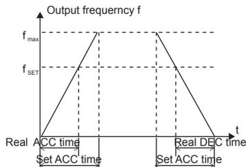
**Figure 6.1 Acceleration and deceleration time**
