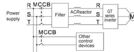
Figure 4.17 Main circuit wiring at input side
