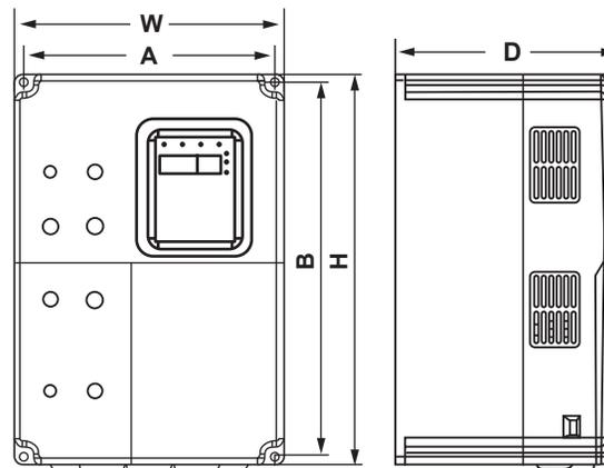
**Figure A-1 Dimensions (15kW and below) (380V)
