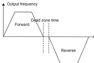
Figure 6.4 FWD/REV dead time diagram.
