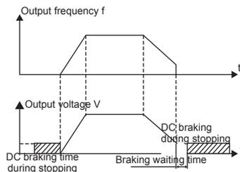
Figure 6.3 DC braking diagram.
