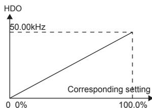
Figure 6.15 Relationship between HDO and corresponding setting.
