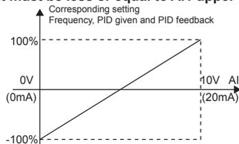
**Figure 6.13 Relationship between AI and corresponding setting.**
