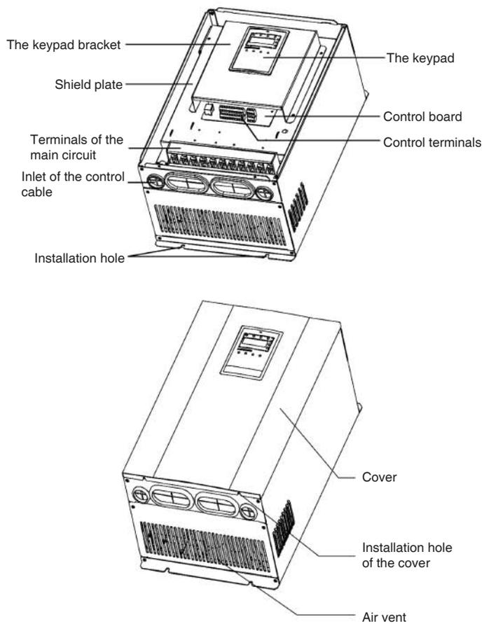
Figure 1-3 Parts of inverter (18.5KW and above)
