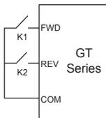
**Figure 6.09 2-wire control mode 1.**
