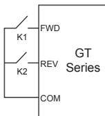
**Figure 6.10 2-wire control mode 2.**
