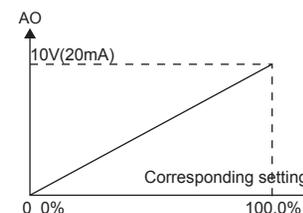
**Figure 6.14 Relationship between AO and corresponding setting.**
