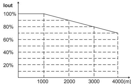
**Figure 3.1 Relationship between output current and altitude**
