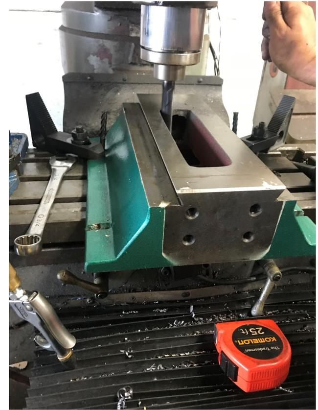
We used a manual mill to do this...because we have one. You may have to use a grinder. You'll be removing however much it takes to get the ball screw in. I wish I could be more precise, but casting are different.
