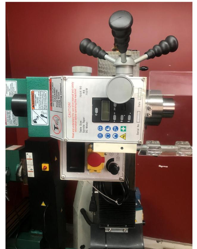
Move the head to the top of the column. Loosen the bolts for the head and rotate it 90 degrees. This will expose the bolts for the lead screw nut in Z. You can also just remove the head. It will make things easier, later
