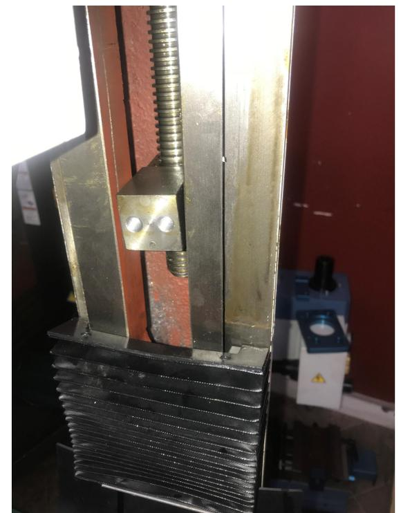
Remove the bolts from behind the head. Screw the lead screw until the lead nut gets to the slot in the column. Take the block off as shown, then you can pull the lead screw out from the top
