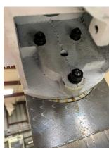
REMOVE THE Z HANDLE. REMOVE THE 4 CAP SCREWS AND PRY OFF THE PLATE WITH A SCREWDRIVER
