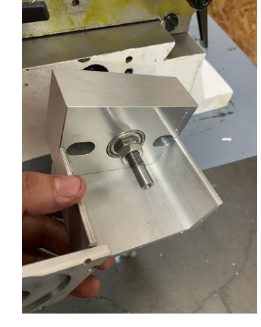
NOW BOLT IT ON TO THE BASE. LEAVE THIS LOOSE AS WELL. NOW I SUGGEST YOU ATTACH A MOTOR TO THE BALL SCREW SO YOU CAN RUN IT BACK AND FORTH AS YOU TIGHTEN IT UP. THE BALL NUT BLOCK AND MOTOR MOUNT HAVE SIDE TO SIDE ADJUSTMENT TO MAKE SURE THERE IS NO BINDING
