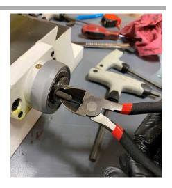
REMOVE THE BOLTS FROM THE PLATE AND DO THE SAME THING YOU DID WITH X. TIGHTEN DOWN THE GIB SCREWS AND TURN THE LEAD SCREW TO PUSH THE PLATE OFF THE BASE
