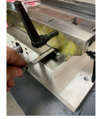
REMOVE THE 1/4" PLATE FROM THE Y ASSEMBLY.
