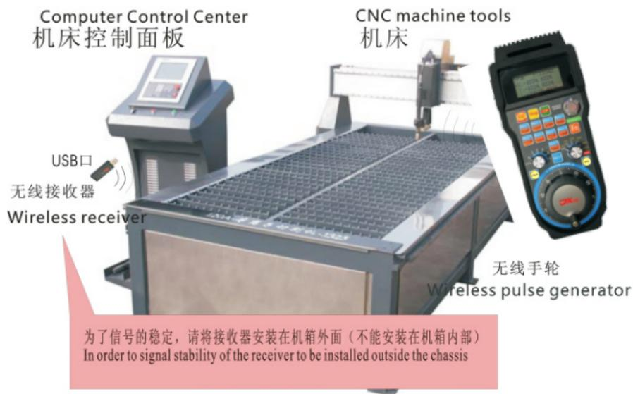
In order to signal stability of the receiver to be installed outside the chassis
