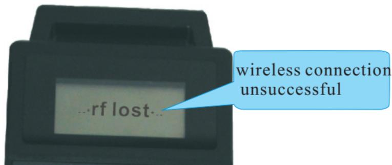
When USB receiver and MPG connect unsuccessfully, For example, USB receiver do not plug into PC, our wireless handwheel will display status like above photo showed)
