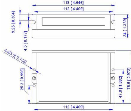
Figure 1: Mechanical specifications
