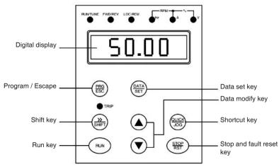
Figure 5-1 Keypad schematic diagram
