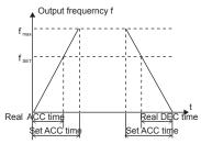
Figure 6.1 Acceleration and deceleration time
