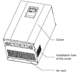
Figure 1-3 Parts of inverter (18.5KW and above)
