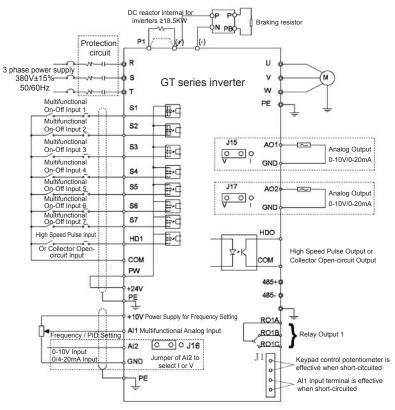
Figure 4-13 Typical of Wiring Diagram
