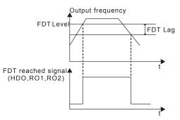
Figure 6.19 FDT level and lag diagram.
