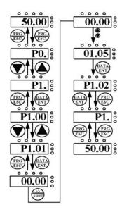
Figure 5.2 Flow chart of parameter setting.
