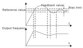
Figure 6.23 Relationship between bias limit and output frequecy.
