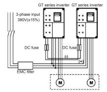
Figure 4.20 Wring of common DC bus.
