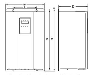
Figure A-2 Dimensions (18.5~110kW) (380V)
