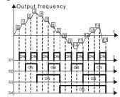
Figure 6.25 Multi-steps speed operation diagram.
