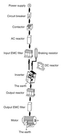
Figure 4-1 Connection of peripheral devices.
