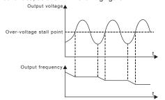
Figure 6.28 Over-voltage stall function.
