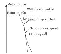
Figure 6.21 Droop control diagram.
