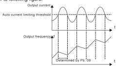
Figure 6.29Current limiting protection function.
